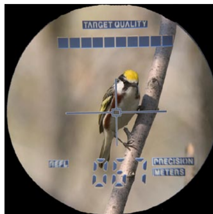
Laser rangefinders were used in training point counters to estimate distances for abundance surveys. This Chestnut-sided Warbler is 67 meters from the observer
